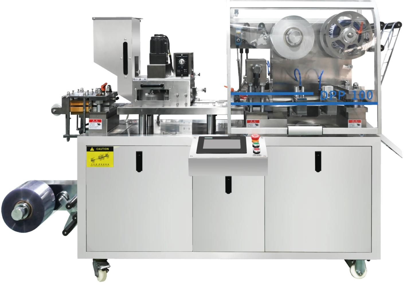
The DPP-100 is an economical automatic blister packaging machine that supports aluminum-plastic packaging using PVC or PVDC aluminum foil. It features a servo drive and PLC control and is designed mainly for small to medium pharmaceutical companies, health supplement makers, and labs. It is suitable for individually sealed packaging of tablets, capsules, gummies, and similar products.
