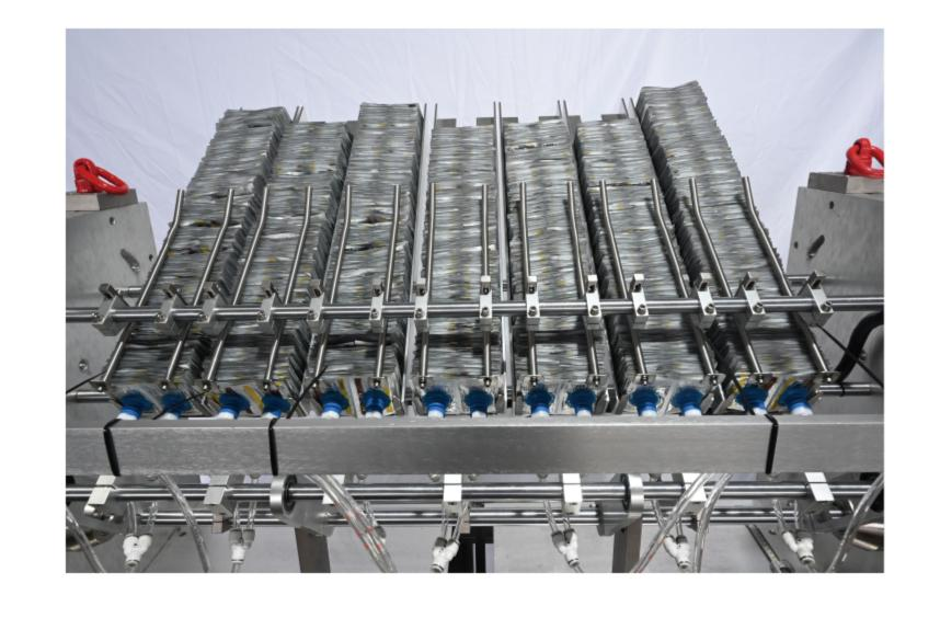
The FTZH-130 fully automatic cartoning machine is an upgraded version, redesigned using the newest technology to greatly improve performance. It can pack up to 120 cartons per minute while remaining stable at high speeds. This machine is ideal for packing medicines (blister packs) or plastic and glass bottles into cartons. It automates the entire process, including inserting instruction leaflets and sealing carton flaps, with optional hot melt glue sealing.
