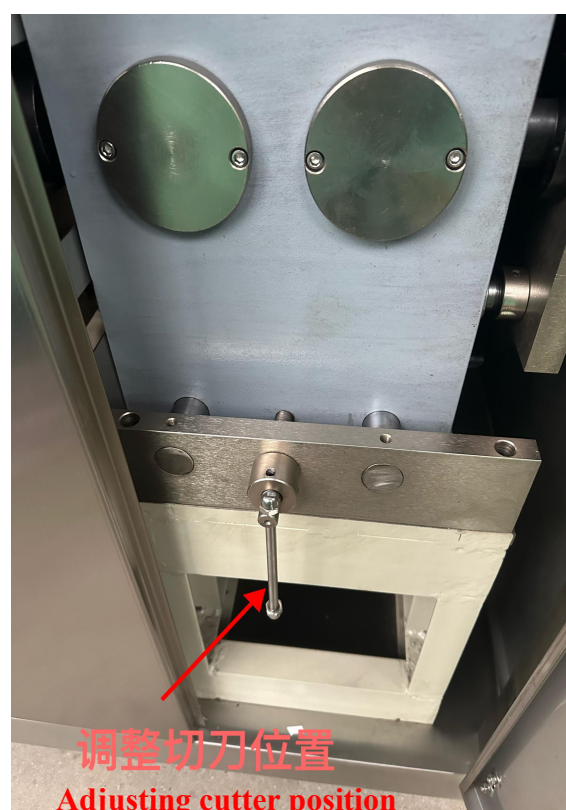
Fig. 4 Adjusting cutter position
