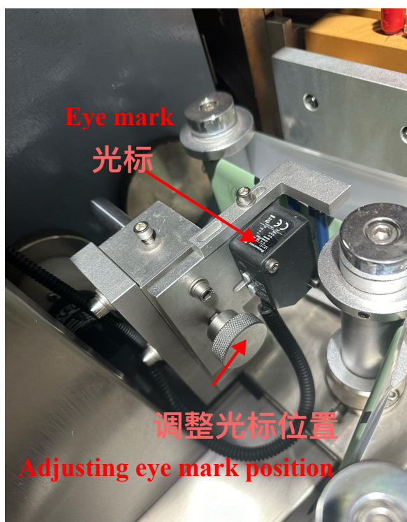
Fig. 1 Adjusting eye mark position
