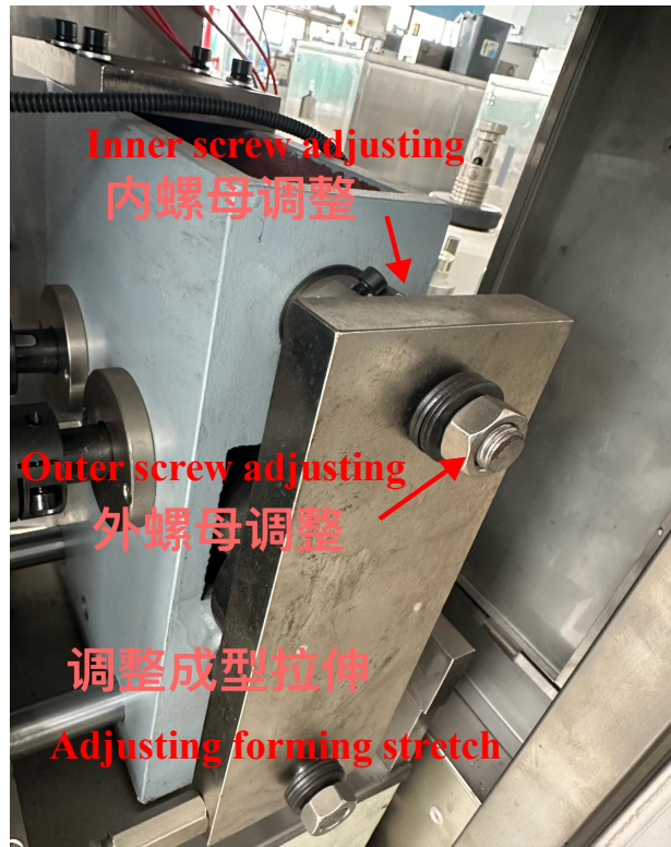
Fig. 6-1 Adjusting forming stretch
