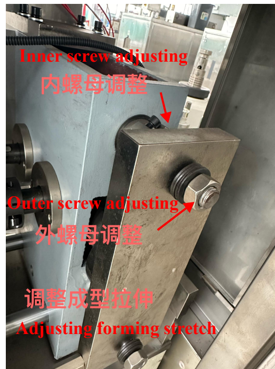
Fig. 6-3 Adjusting forming stretch
