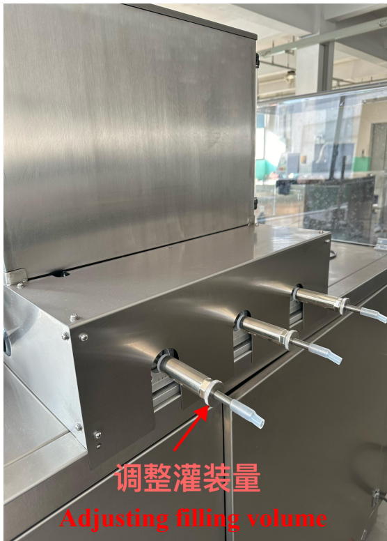
Fig. 5 Adjusting filing volume
